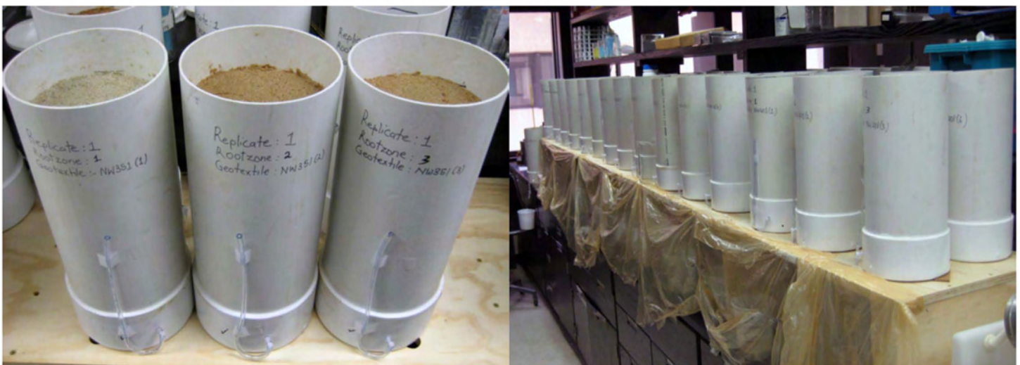
Figure 6. Columns used to measure potential clogging of geotextiles by fines migrating out of the root zone.
